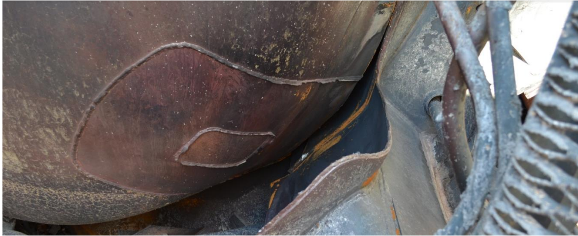
Pad-to-tank Weld Separation, Car ADMX 31172, Tiskilwa, IL Derailment ( FRA Photo via NTSB Docket )
