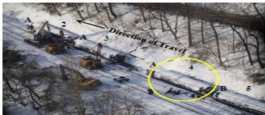
Figure 3: Resting positions of CBTX 742201 (02), CBTX 742774 (03), CBTX 742792 (04), and GATX 286285 (05).
